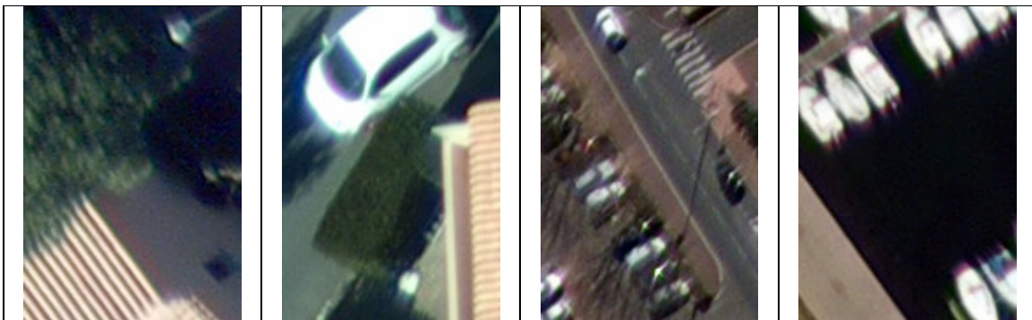
Fig. 6. Consequences of the use of off-the-shelf lenses with the UCD on the geometric quality in the corners of images. From left to right : lower-left corner (GSD : 5cm), upper-left (GSD : 5cm), upper-left (GSD : 20cm), upper-right (GSD: 20cm)
