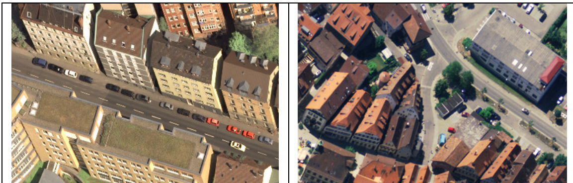
Fig. 7. Field of view cross track of 69.3^\circ for DMC on the left and 62^\circ for ADS40 on the right leads to numerous occluded areas on the borders of the images.
