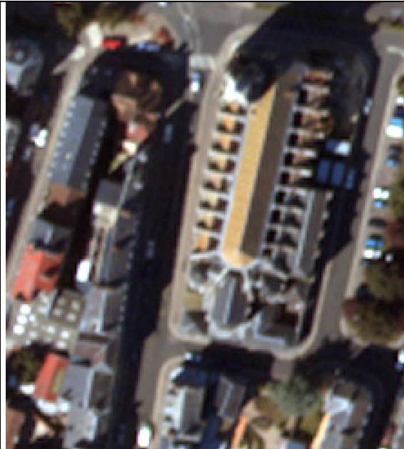
Fig. 1b : extract of the initial GSD 68cm image re-sampled to 40 cm (bicubic re-sampling)
